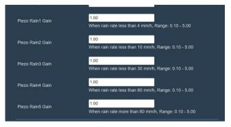
Figure 10: Set five rain gain parameters
