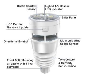
Figure 2: Sensor package assembly components
