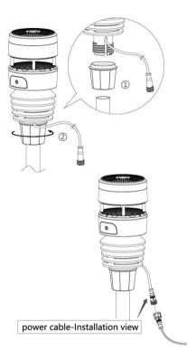
Figure 5: Sensor package mounting diagram
